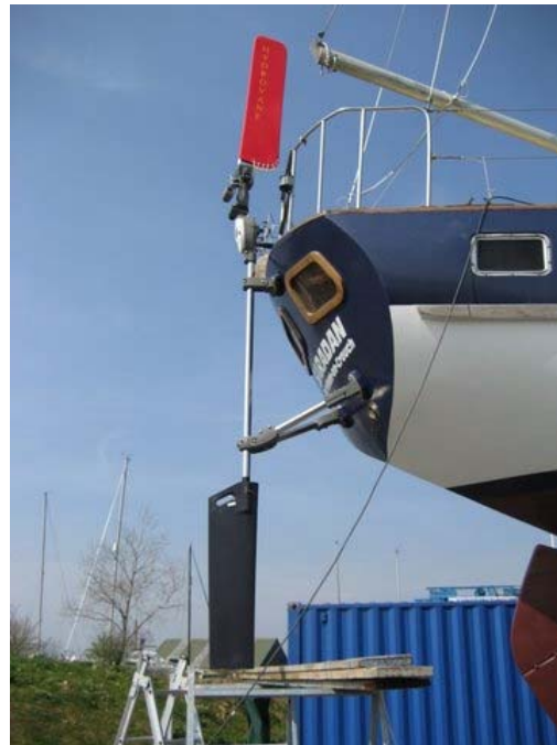
ENDURANCE 45 – 25 tons complete assembly is 13 to 15 feet (3.9 to 5m.) high
