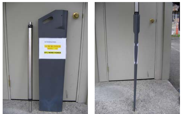
New Rudder – 43.5" (1,105 mm) Tall – Blade 1.5" (38 mm) at its thickest True 'NACA' Profile – Negligible Drag
